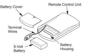
Figure 39 - Installing Alkaline Battery in Hand-Held Remote Control Unit
